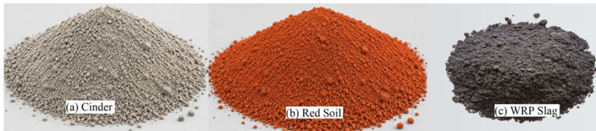
Fig. 1. Source materials: (a) red soil, (b) cinder and (c) waste-recycling-plant (WRP) slag. Photographs were recovered from the supplied experimental presentation.
