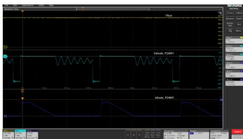
Fig. (4). P24M1 Diode Voltage and Current at Maximum Load
