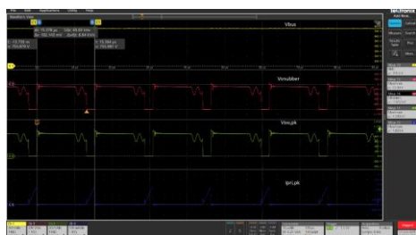
Fig. (6). Snubber Voltage, Switching Voltage and Primary Current at Nominal input Voltage of 760V
