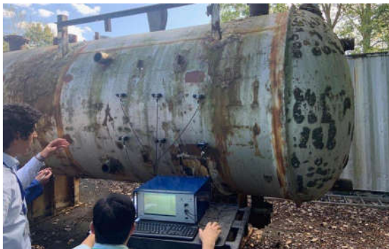
Fig. 16. AE Sensors are Attached at The Surface
