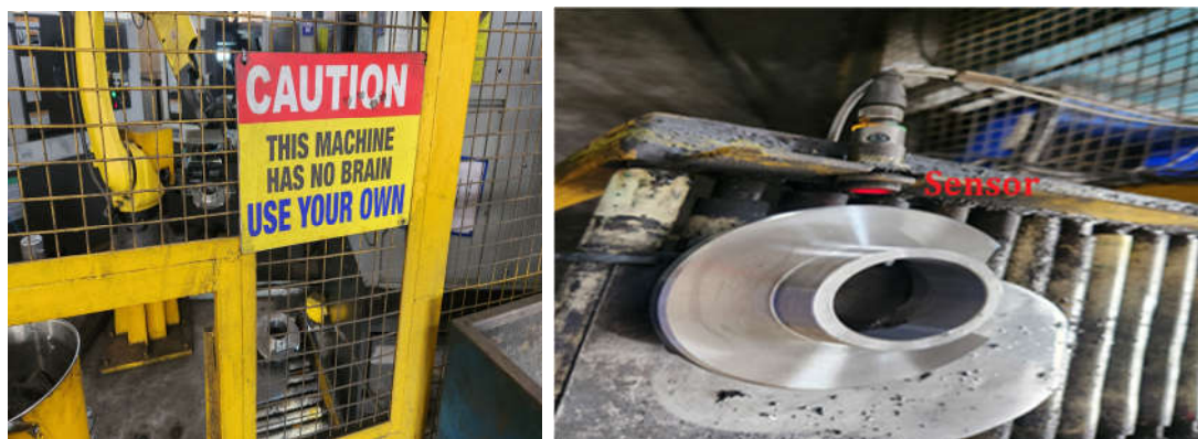
Fig.7 Conveyor sensor used if conveyor full with parts sensor detect that and then robot not kept parts on conveyor.
