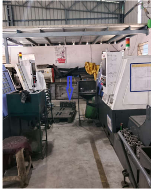
Fig.2 Manual machining layout with congested workspace, poor material flow, and operator-dependent handling causing motion waste and ergonomic issues.
