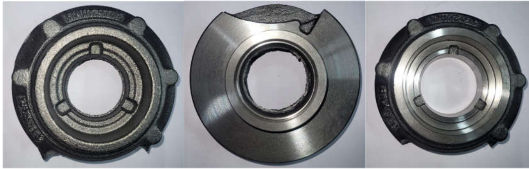
Fig. 1 Photographic view of component (As cast, First Side machining, Second Side Machining)
