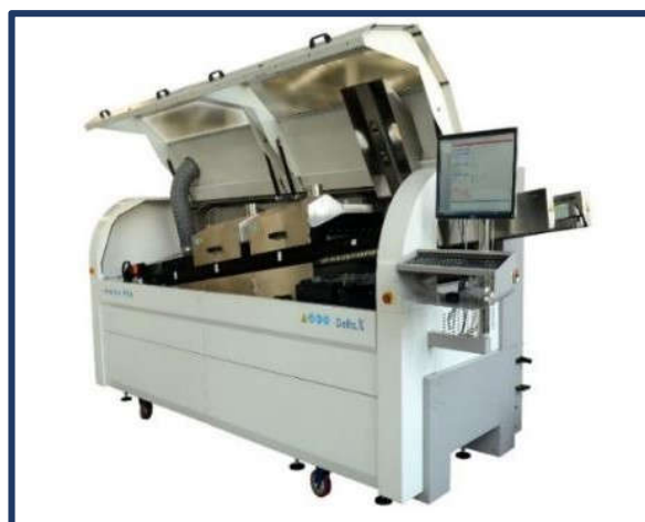
Figure 2. Wave Welding Machine (DELTA X example). Representative wave welding machine used as a case study for reliability and predictive maintenance analysis [10].
