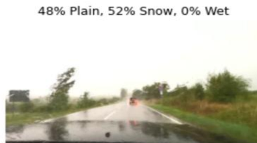
Figure 10. Incorrect Classification for Wet/Slurry Roads
