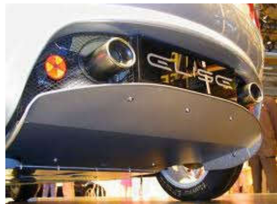
Fig.1. New Elise diffuser without intermediate ribs
