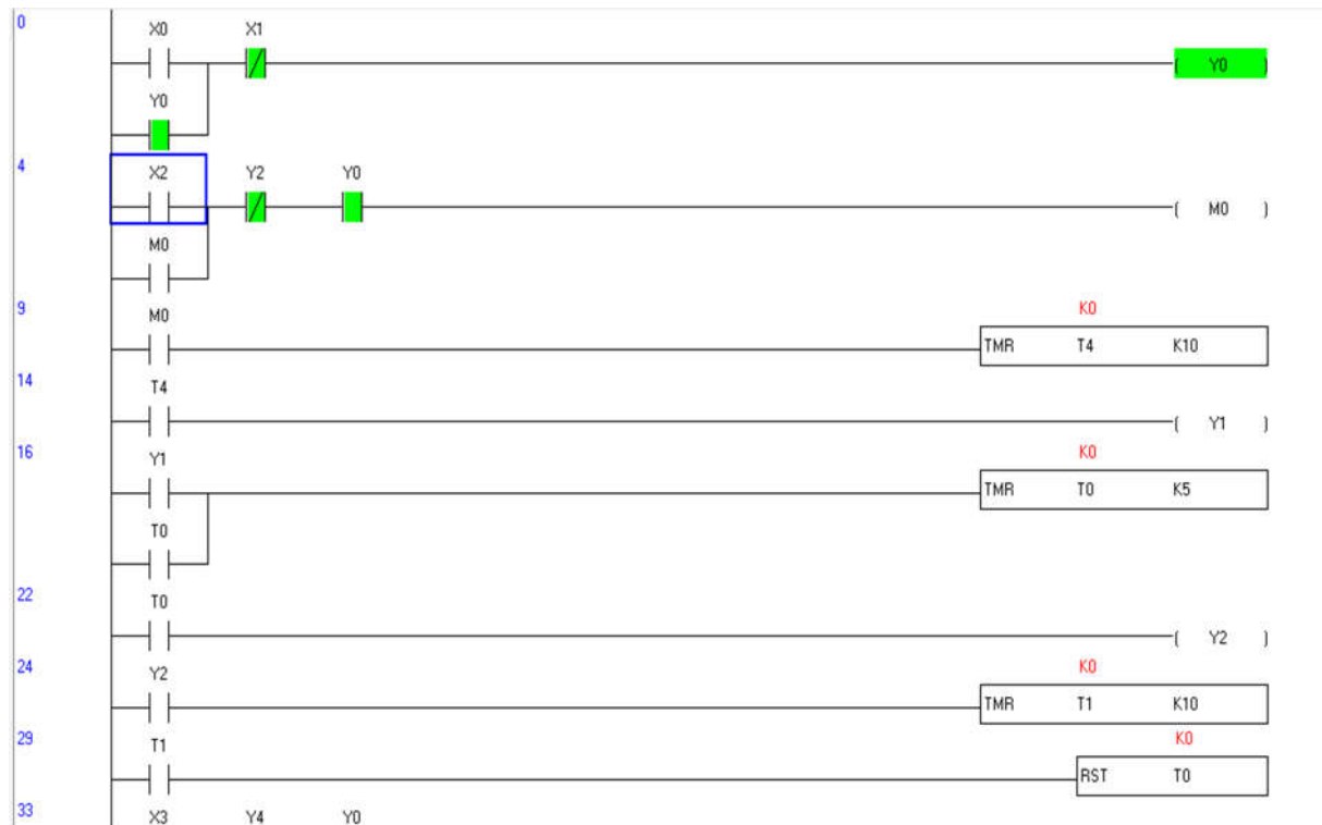
Figure 10. Logic for Crushing System
