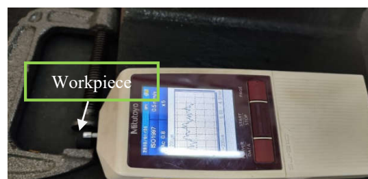
Figure 4. Measurement of surface roughness
