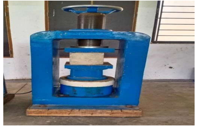
Fig 4.5 Polymer Concrete Cubes after Compression Test 4. RESULTS AND DISCUSSIONS
