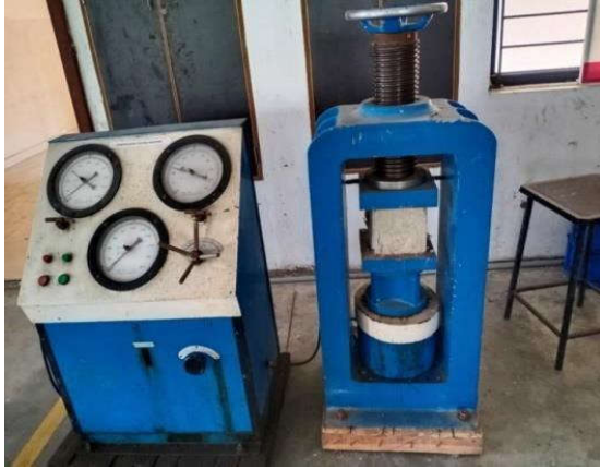
Fig 4.5 Polymer Concrete Cubes after Compression Test 4. RESULTS AND DISCUSSIONS
