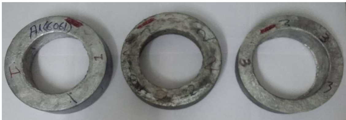
1 2 3 Figure 2. Al (6061) as cast and FGMCC rings
