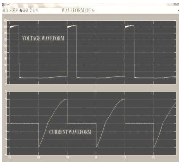
Figure 7: Output waveform of switch S 2
